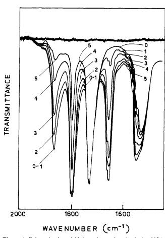
Figure 1. Polymerization of  $N^{\epsilon}$ -benzyloxycarbonyl-L-lysine NCA in dioxane initiated by sodium hydride. Infrared spectra recorded at various reaction times: initial (spectrum 0); 20 min (spectrum 1); 45 min (spectrum 2); 70 min (spectrum 3); 100 min (spectrum 4); 130 min (curve 5). The monomer to initiator molar ratio was 12.5.
